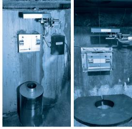
Telelot VDD2v4 systems tailored for measuring the dam's horizontal deformations. These enhancements mark a substantial improvement in monitoring capabilities, ensuring the safety and efficiency of the Sardar Sarovar dam in India.
